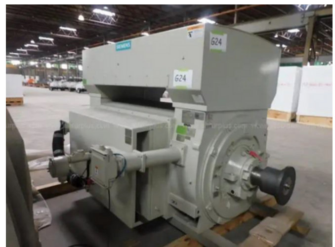
Unused Siemens 6,500 HP Electric Motor
